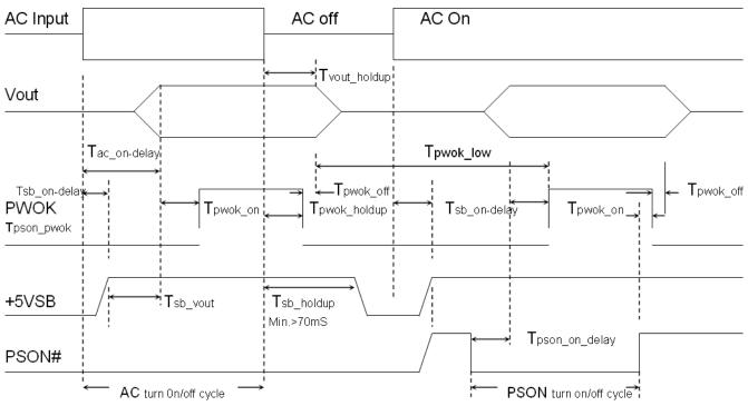
Figure 2: Turn On/Off Timing
